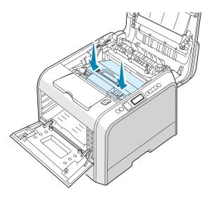
**14** Firmly push the lock levers on each side towards the top cover, as shown below, to lock the transfer belt into place.
